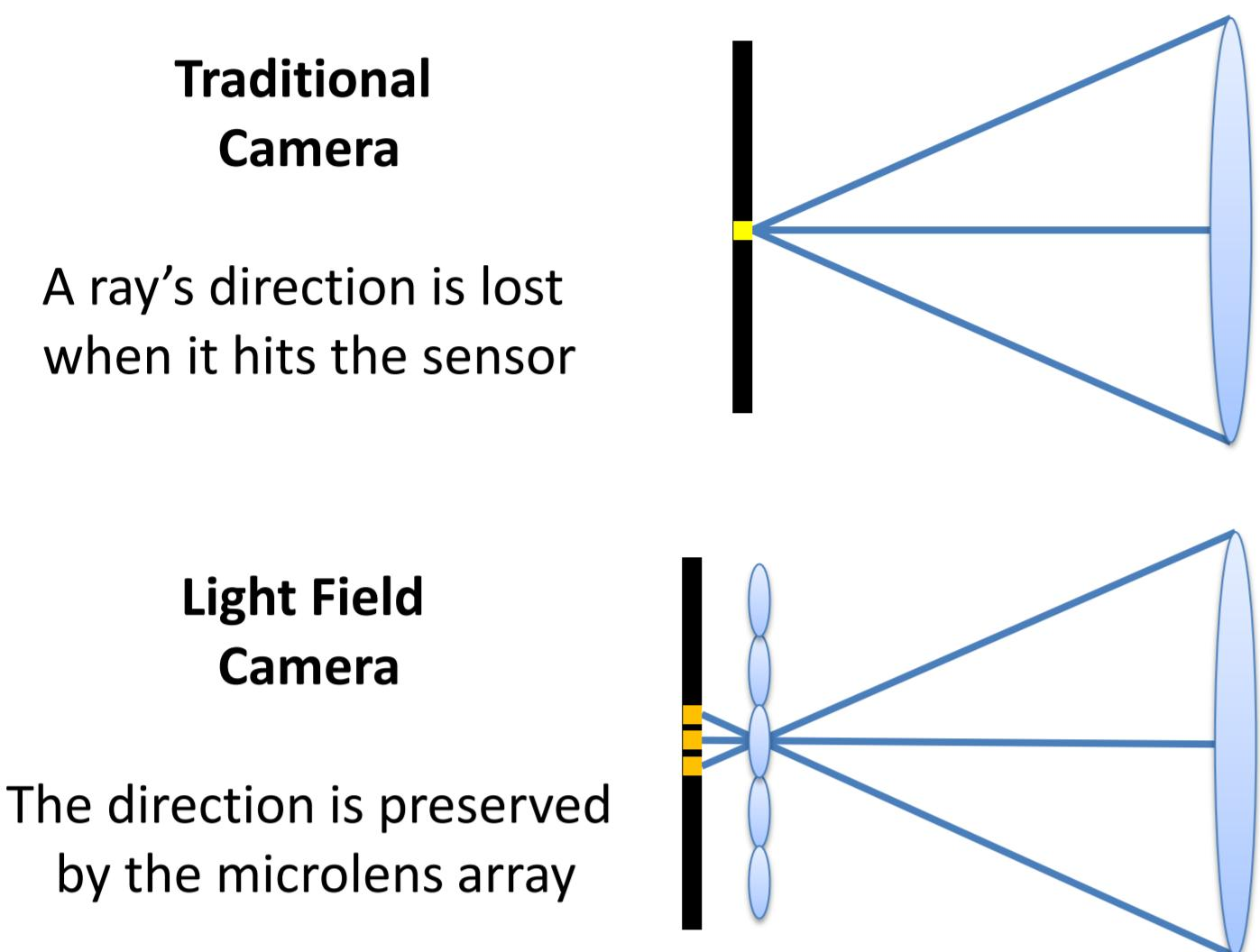
A **light field camera** **captures 3-D data** from a single image. This is because a **microlens array**, consisting of thousands of tiny lenses, splits rays coming from different directions onto different pixels. Knowing a ray's intensity and direction means from a single raw image we can **digitally refocus, change viewpoint, aperture, and estimate depths** within a scene. These abilities come at the expense of spatial resolution.
