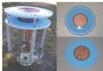
N. Gagnon, A. Petosa, "Using Rotatable Planar Phase Shifting Surfaces to Steer a High-Gain Beam," IEEE Trans. Antennas Propag., Vol. 61, No. 6, June 2013
