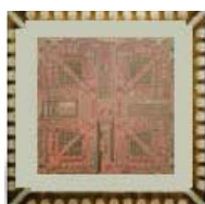
64 Element Ka-Band Array Using Anokiwave Quad Core Tx SATCOM IC
