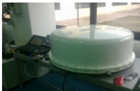
Ka Band railway radome under test by using KASATSatellite
