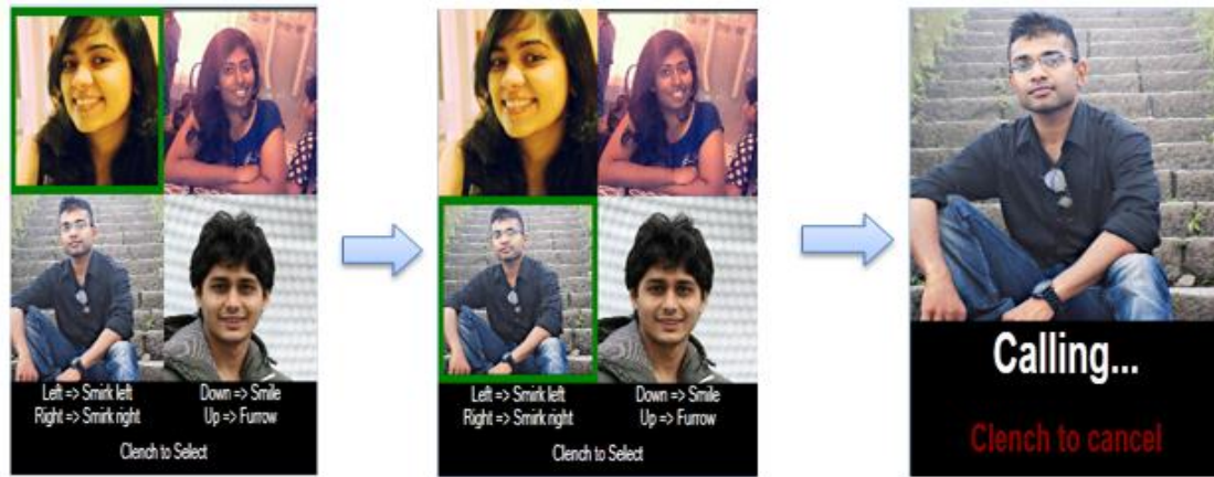
Figure 3: Skype Dialer. Smirk left, Smirk right, Smile and Furrow are used to navigate through the various contacts on the dialer. Clench is used to connect to the selected contact and also to disconnect an ongoing call.
