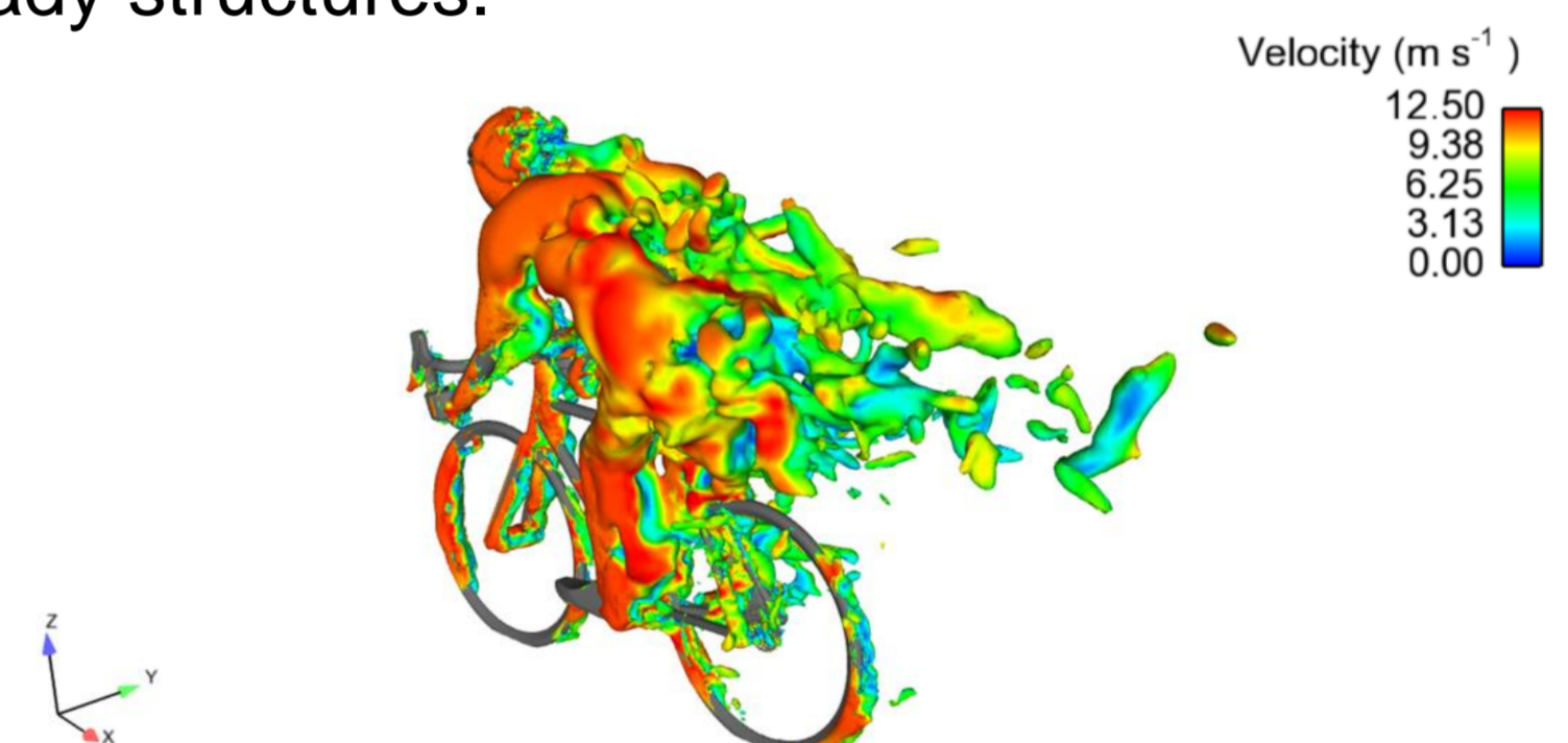
Fig 4 Isosurface of the instantaneous pressure at 15° yaw angle (DES)
