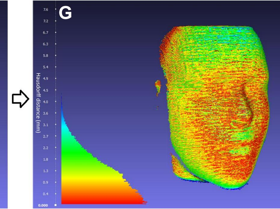
**Registration:** 3D imaging systems can be used to produce a point cloud of the head: a set of data points comprising the coordinates at which the surface has been measured by the system. This can be done using structured light (used here, [3]) or time-of-flight systems. The resulting point cloud must then be registered with preoperative images.
