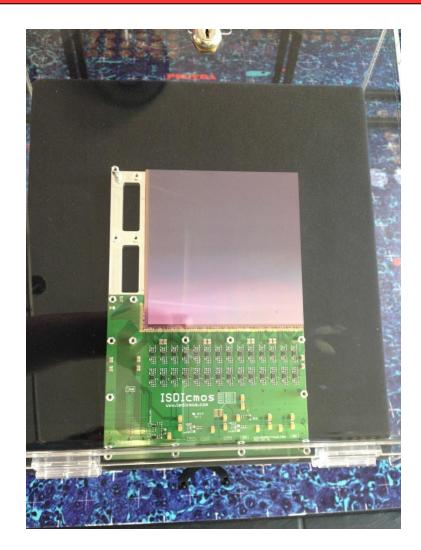
50x50 micron pitch, 14micron thick
