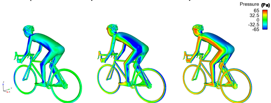
Figure 6: Pressure distribution on the surface of the cyclist in different crosswind yaw angles of the RANS standard k-\epsilon turbulence model: (a) \beta = 0^\circ , (b) \beta = 45^\circ and (c) \beta = 90^\circ .
