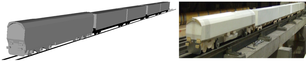
Figure 1: Comparison between train models used in the numerical and physical experiments
