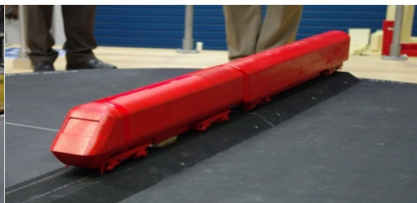
Figure 2: 1/25 th scale HST windtunnel model.
