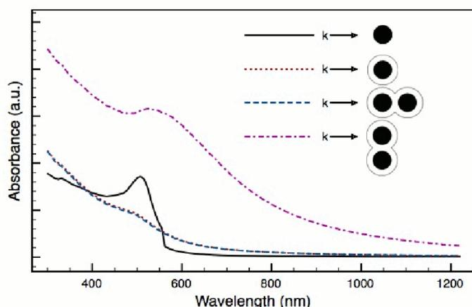
DDSCAT calculations for isolated Au and Au(core)Pd(shell) spheres compared to Au(core)Pd(shell) particles oriented with conjoining axis parallel and perpendicular to light (k). Au and Pd are represented in the schematics by black and white, respectively.
